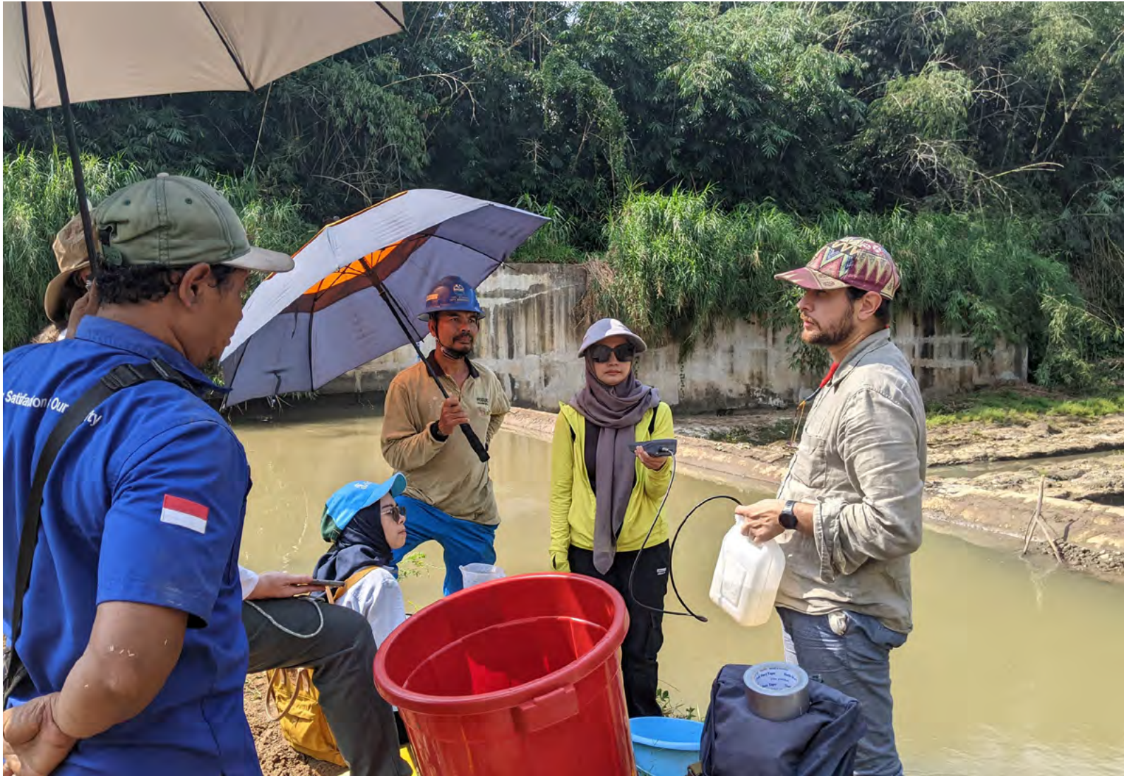
Indonesia — PDAM Semarang and Short Term Expert Ivar Abas are preparing a river flow measurement (salt dilution method) for the development of a new water treatment plant in Jatisari.
