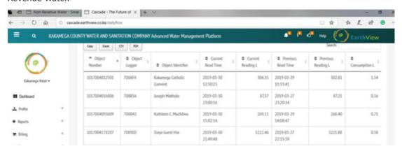
Above: A screen shot of the smart meter readings that are transmitted after every hour. KACWASCO has a tower that transmits the readings every hour.
